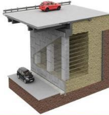
Mixed Abutments Spans over 40m
